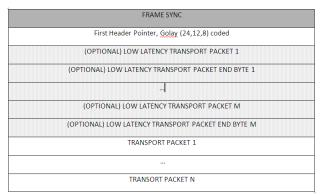
**Figure 2 - Transport Frame Structure**
