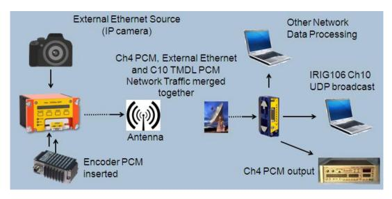
The following diagram illustrates the ground segment architecture.
