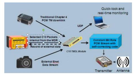
Figure 9 - Merging of External PCM and Ethernet into C10 TMDL Stream
