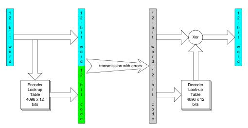
Figure 3 - Extended Golay Encoding and Decoding
