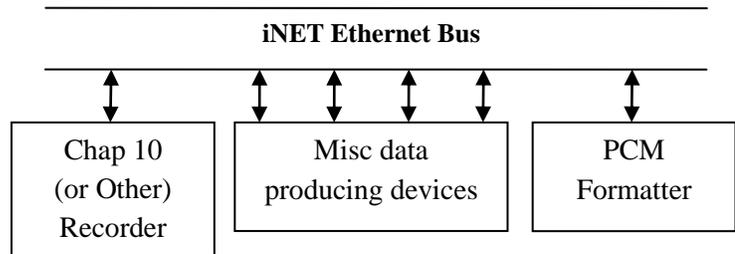
**Figure 6 Notional iNET Centric Architecture**
