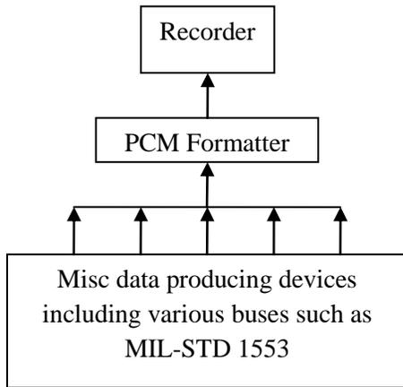
**Figure 5 Notional Traditional PCM Centric Architecture**
