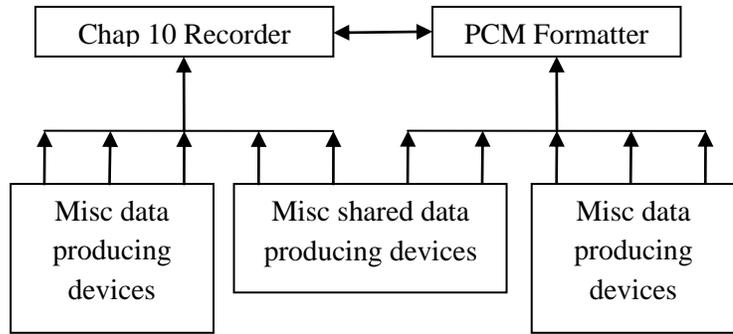
**Figure 4 Notional Chapter 10 Centric Architecture**
